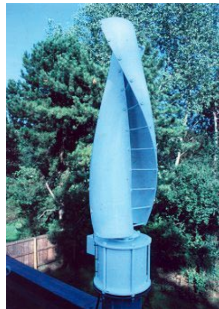
A vertical axis wind turbine.
